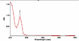
Figure 3. UV VIS standard spectre for niacin
