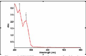
Figure 1. UV VIS standard spectre for thiamine
