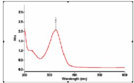
Figure 5. UV VIS standard spectre for trans-retinols
