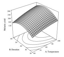
**Figure 1.** Response surface plot showing the effect of temperature and duration on melanin extraction from black tea leaves. The liquid-solid ratio was constant at 100 ml/g
