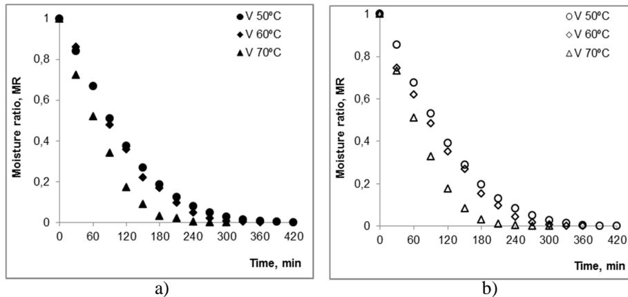
**Figure 2.** Influence of temperature and time on the MR of pumpkin during vacuum drying: (a) cylinder shape, (b) cube shape
