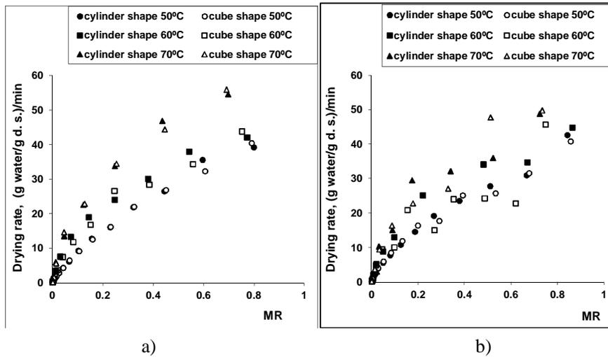
**Figure 3.** Effect of drying air temperature and moisture ratio on the drying rate of pumpkin samples: (a) convective air drying, (b) vacuum drying
