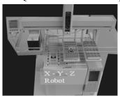
Figure 1 Three-dimensional automated system for the injection of samples AOC-5000 (GCMS-QP2010xAOC-5000)
