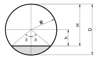
volume of charge and the inside volume of the drum, or aria of cross section of the charge  $^{A}inc$  and aria of cross section of the drum  $^{A}t$  (fig.1) [5].
