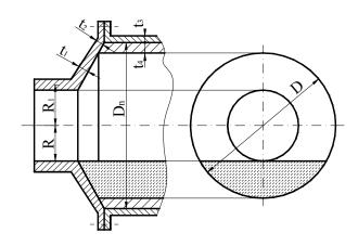
Fig. 2. Scheme for determination of the tubular trunnion radius in the inlet.
