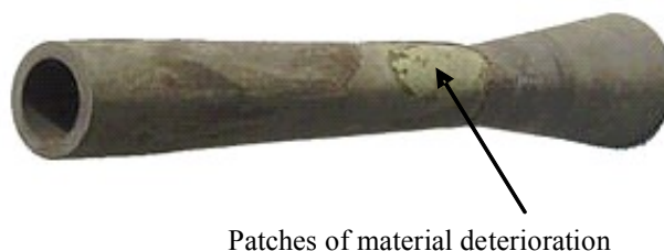
Fig. 1. The conventional WC-Co blasting nozzle used in thermo-abrasive blasting with signs of material deterioration due to the excessive heat.
