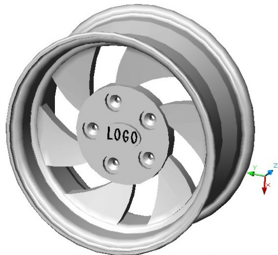
Figure 10: The rim of easy alloy with 6 spokes (curves section)
