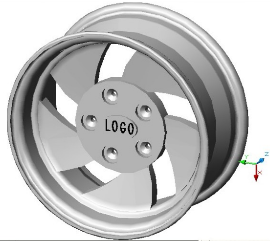
Figure 9: The rim of easy alloy with 5 spokes (curves section)
