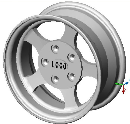
Figure 12: The rim of easy alloy with 5 spokes (cylinder interior tangent section)
