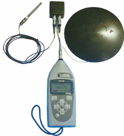
Fig. 2. MAESTRO vibrometer and 01dB triaxial seat-pad accelerometer
