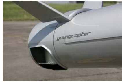
Fig. 4. NOTAR system used by NEO helicopter from YoungCopter [14]
