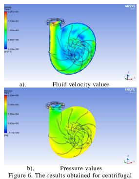
pump analysis, model 3,  $(\alpha < 90^{\circ})$
