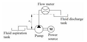
Figure 1. Schematic representation of pump operation
