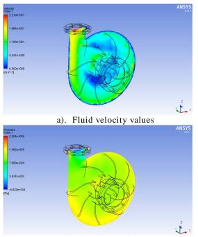
b). Pressure values Figure 4. The results obtained for centrifugal pump analysis, model 1,  $(\alpha > 90^{\circ})$
