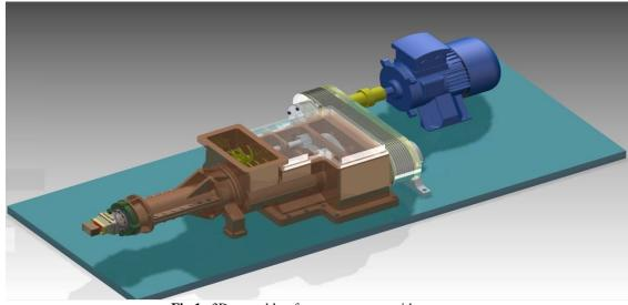
Fig.1 3D assembly of a vacuum press with worm
