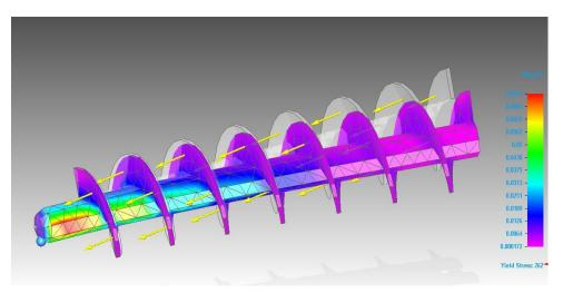
Fig.7 Simulation sketch of tension on spiral worm
