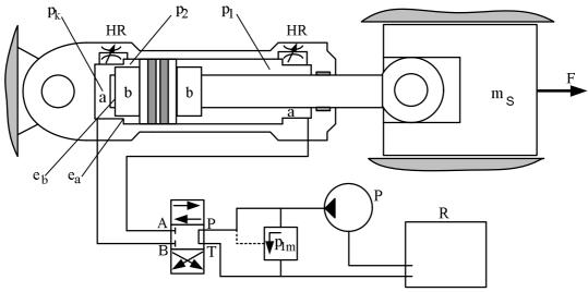
Fig. 1 The work scheme of a hydraulic cylinder fitted with impact cushioning at both ends
