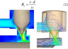
Fig. 3 Adjustable hydraulic resistance
