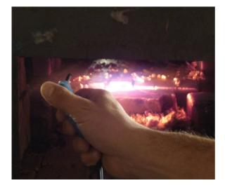
Figura 5. Flue gas analysis in experimental furnace.
