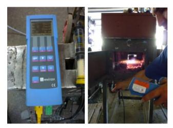
Figure 4. Combustion gas analyzer MINILYZER 02.
