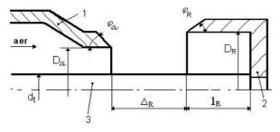
Fig.3. The dimensional scheme of air-jet stem generator
