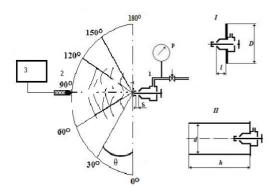
Fig.4. Pattern of performing acoustic measurements of air-jet stem generator at different emission angles: 1- air-jet generator; 2 - microphone; 3 - acoustical measurement system (Solo 01dB-METRAVIB device & Laptop);  $\theta$  - angle of measurement; *I* - air-jet stem generator with reflective disk; *II* - air-jet stem generator into cylindrical glass tube.
