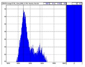
Fig.7. Acoustic spectrum of air-jet stem generator: resonator distances  $\Delta$ =1.2 mm and supply pressure p =0.1 MPa.
