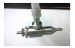
Fig.2. Experimental air-jet stem generator with variable resonator distance
