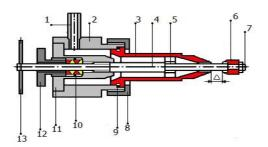
Fig.1. Experimental air-jet stem generator with variable resonator distance: 1- air connecting pipe; 2-base; 3-nozzle; 4-stem; 5-cross support;
