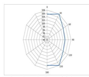
Fig.6. The angular diagram of air-jet stem generator with reflector disk: resonator distances  $\Delta$ =1.2 mm and supply pressure p =0.1 MPa.
