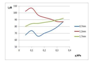
Fig.5. Overall intensity levels of air-jet stem
