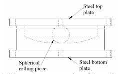
a) Schematic representation of the rolling pendulum isolation system
