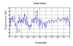
Figure 4.4. Transfer function for the vertical direction of movement
