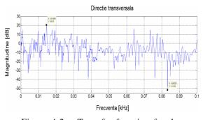
Figure 4.2. Transfer function for the transversal direction of movement
