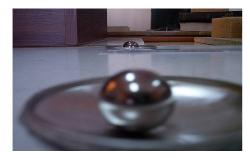
Figure 3.2. Reduced scale model of the rolling pendulum isolation system
