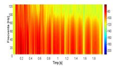
(a) Pier frequency spectrogram over time
