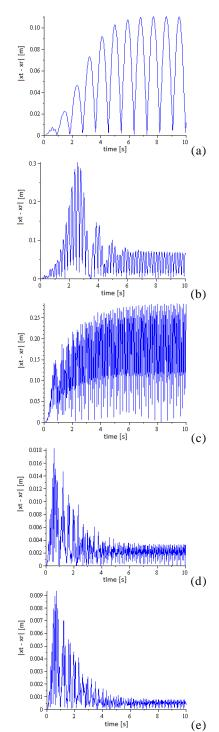
Fig. 1. The instantaneous absolute differences between evolution of theoretic and realistic displacements during the first ten seconds of transitory state for an SDoF dynamic system. The cases have the following signification
