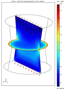
Fig. 2. Distribution of strain energy density (color map) and heat flux (arrows field) within the orthogonal sections of a profiled cylinder isolator
