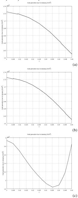
Fig. 4. Steady state evolutions of the heating due to damping parameter along the longitudinal axis of the elastomeric element. The cases have the following signification
