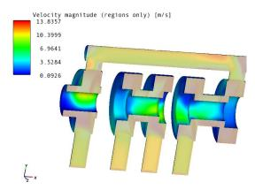
Fig. 5. The graphic result of the simulation flow for a directional valve.
