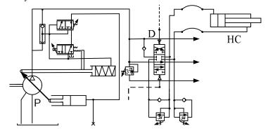
Fig. 1. Partial hydraulic diagram of a hydraulic excavator
