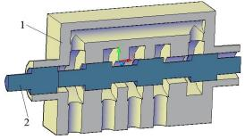
Fig 3. Directional valves DN20. 1- hausing; 2 – spool.
