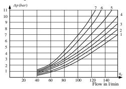
Fig. 3. Pressure drops on different connecting routes (2 - P / A, 4 - A / T, ... ) depending on the flow of hydraulic fluid.
