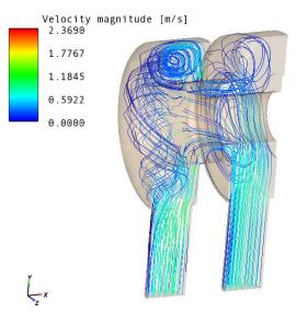
Fig. 6. Lines of flow in the body fluid.
