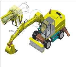
Fig. 2 The 3D Model of the excavator rotating arm
