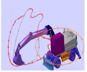
Fig. 10. Access areas of the excavator bucket
