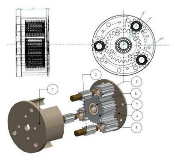
Fig.5. Subassembly of planetary gear
