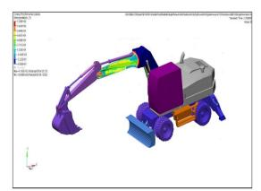
Fig. 8. Modeling arm no.2 after meshing
