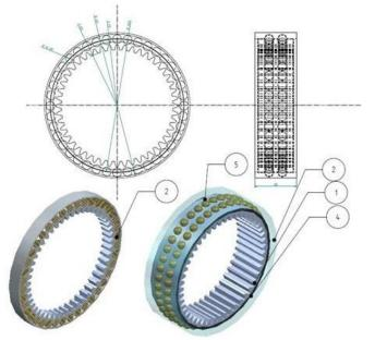
Fig.4. Subassembly of special radial-axial bearing
