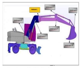
Fig.6 The modified joining of the excavator arm
