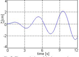
Fig.7. Time evolution of the boom motion
