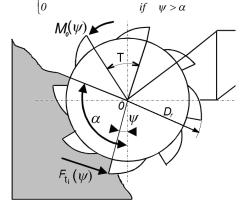
Fig.4. Schematic diagram for cutting force The notations from Eqns. (3) and (4) have the following significances:  $\Psi$  - the angular
