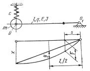
Fig.6. Simplified dynamic model of the boom
