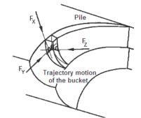
Fig.3. Digging forces at the bucket wheel
