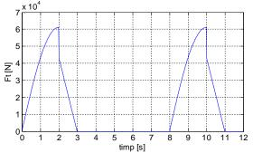
Fig.5.Cutting force simulation for a single bucket
