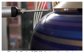
Fig. 5. Probe 55R42 during the velocity measurements
