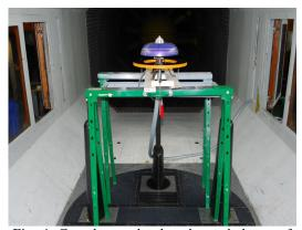
Fig. 4. Coanda nozzle placed on a balance of INCAS low speed wind tunnel
