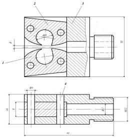
Figure 2. The experimental air-jet sonic generator with two resonators: 1-housing, 2- top resonator, 3- bottom resonator, 4- mounting pin,  $\delta$ - generator slot
