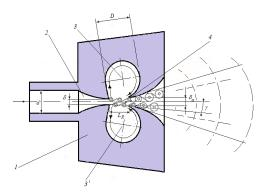
Figure 1. The flow scheme of sonic generator with two resonators : 1-base; 2-convergent nozzle; 3,3'-resonance cavities; 4-resonator edge; D-resonance cavity diameter;  $\delta$ convergent nozzle slot;  $\delta_a$ - generator slot; L<sub>R</sub>resonator neck length; d-inlet port diameter
