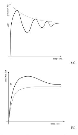
Fig.3. The change in pressure valve (analytical solution)
