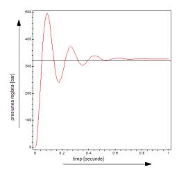
Fig.1. The variation of the pressure on the valve adjusted pressure
