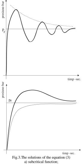
b) supercritical and critical operation
