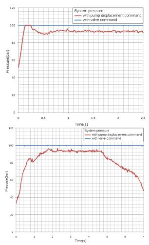
Fig.2. Dynamic response of pressure in hydraulic volumetric units (experimental analysis); ordered - presume ( bar); basis- time (sec).
