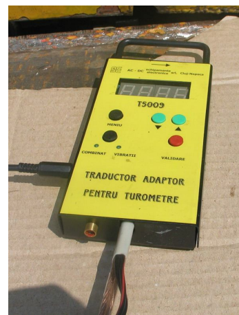
Figure 6 Electronic tachometer T5009 used for the MMT45 engine speed measurement
