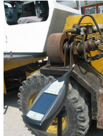
Figure 5 Hand-held analyzer Brüel & Kjær 2250 used for noise level measurement
