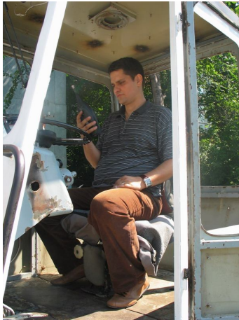
Figure 3 Global sound intensity level measurement inside the cabin of MMT45
