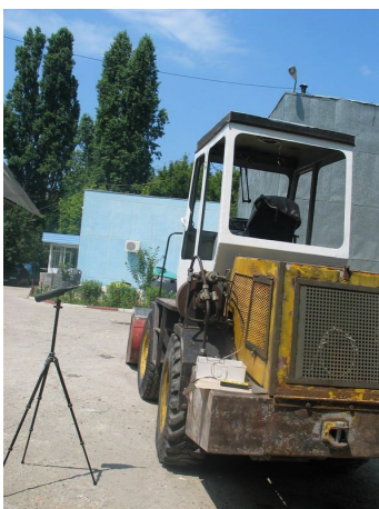
Figure 4 Sound intensity level measurement around the frontal loader MMT45
