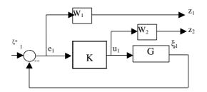
Fig. 4. Specific H<sub>2</sub> design architecture
