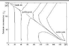
Fig. 1. Phase plane of CSTB with recycle stream
