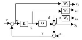
Fig. 3. The H<sub>2</sub> controller design architecture
