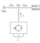
Fig.3. Shunt active power filter with voltage source inverter
