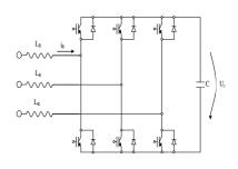
Fig.1. Three phase voltage inverter
