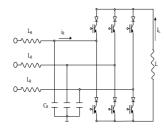
Fig.2. Three-phase current inverter
