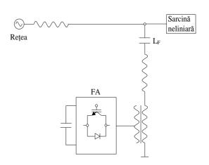
Fig.13. Active power filter in series with shunt passive filter
