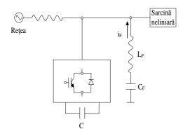
Fig.12. Shunt active power filter and shunt passive power filter
