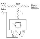
Fig.9. Shunt active power filter with 4 wires and median point on capacity
