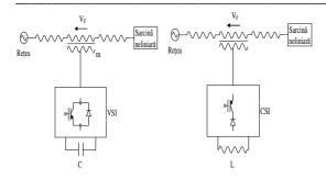
Fig.5. Series FAP - Fig.6. Series FAP -current voltage source source inverter inverter
