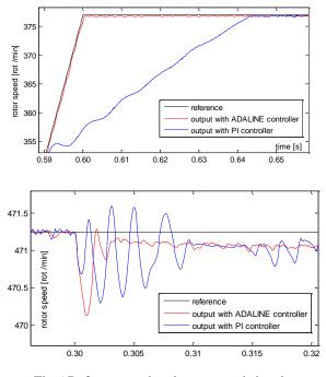
Fig.6 Reference and real rotor speed signals (magnified)
