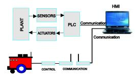
Fig.5. Distributed control structure that includes a mobile robot
