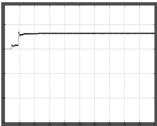
Fig.6 (a) PI controller response under source disturbance condition at 9.1msec
