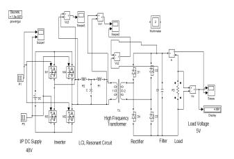
Fig. 5. LCL Resonant DC-DC Converter
