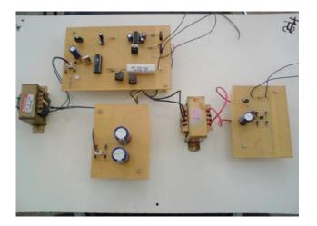
Fig. 10. Embedded controlled full bridge LCL resonant converter. (Hardware Layout)
