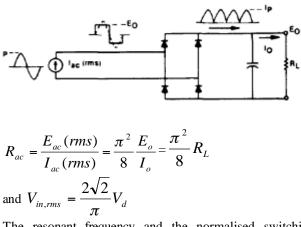
The resonant frequency and the normalised switching frequency is defined as
