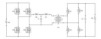
Fig. 3. LCL Series-Parallel Resonant DC-DC Converter.
