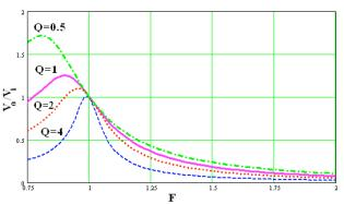
Fig.4. Frequency response of the LCL resonant tank
