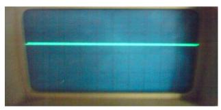
(e) Output of DC-DC Converter. (Load Voltage)
