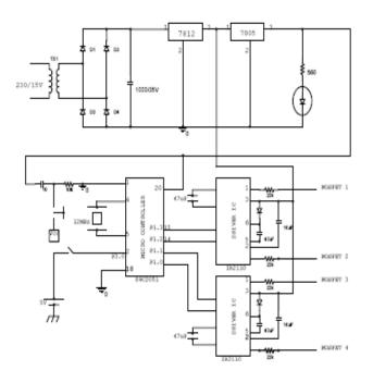
Fig. 11. Control circuit for generating the Driving Pulses.
