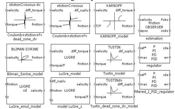
Fig.2. The Simulink® toolbox for friction model and control
