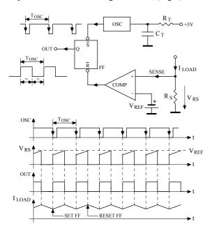
Fig.3. Load current control.
