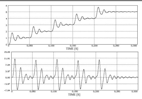
Fig.18. The position and the angular speed for command with constant frequency.
