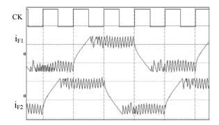
Fig.14. The phase currents in normal drive mode, the inhibit chopping (0.4A/div., 5ms/div.).
