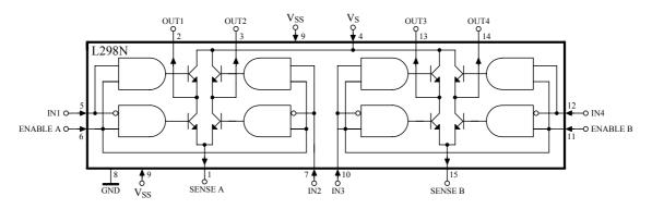
Fig.2. Block diagram of the L298N dual H-bridge driver.
