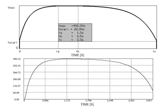
Fig.20. Prescribed speed profile and real speed profile.
