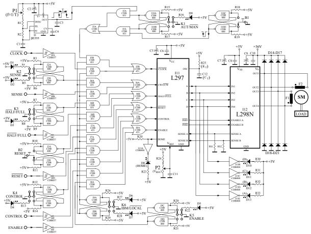
Fig.7. Electrical schematic of the control system. The command signals for the controller L297 are generated through an IBM-PC486 interface (Băluță,
