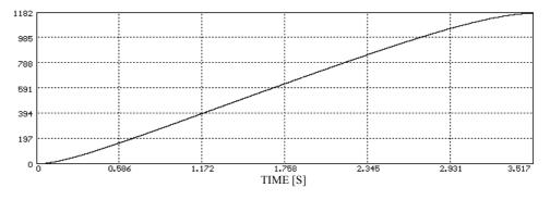
Fig.19. The position for command with exponential profile.
