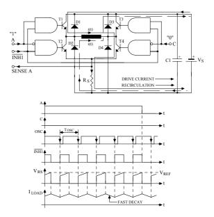
Fig. 5. Inhibit chopping.
