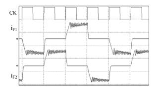
Fig.15. The phase currents in wave drive mode, the phase chopping (0.4A/div., 5ms/div.).
