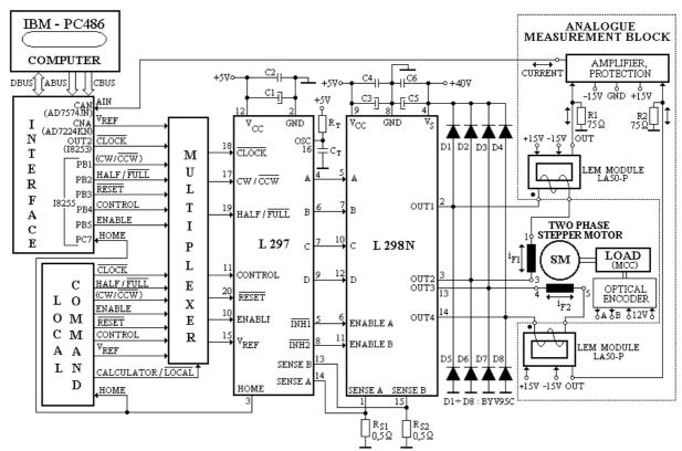
Fig.6. Block diagram of the control system.
