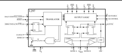
Fig.1. Block diagram of the L297 stepper motor controller.
