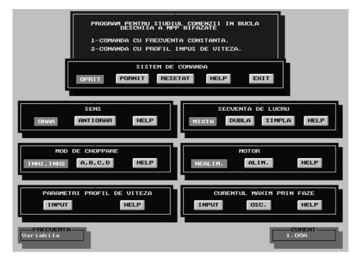
Fig.9. The main menu of the command program. Due to the graphical interface, even a less prepared user can supervise the main parameters of the drive
