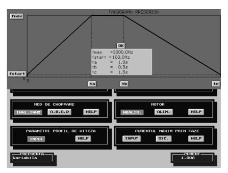
Fig.16. Linear profile of the prescribed velocity.
