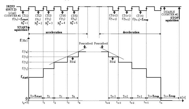
Fig.10. The algorithm that generates the command pulses for the linear speed profile.
