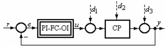
Fig. 1. Structure of fuzzy control system.
