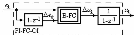
Fig. 2. Structure of PI-fuzzy controller with output integration.
