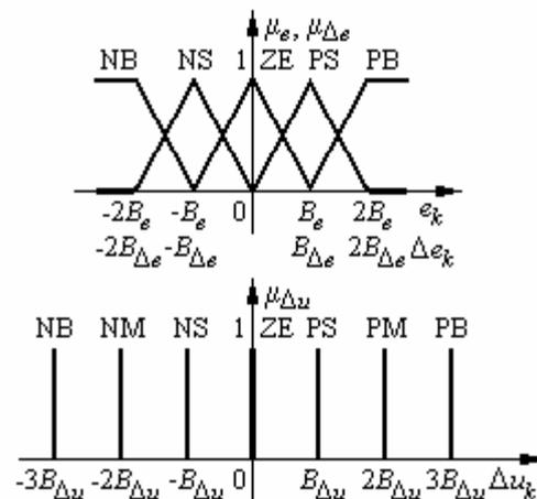
Fig. 3. Membership functions of input and output linguistic variables in B-FC.
