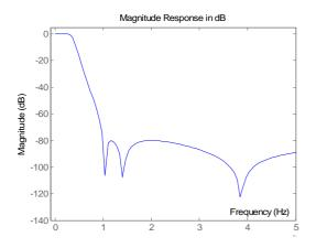
Fig.3. Chebyshev Lowpass filter characteristic.
