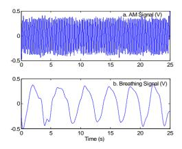
Fig.4. Time-signals after low-pass filtering.
