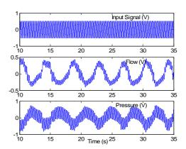
Fig.2. Input and Output Signals for 5Hz.
