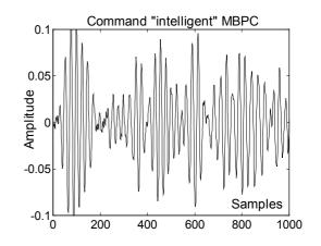
Fig. 9. Controller output u(t) for *intelligent* MBPC
