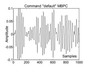
Fig. 8. Controller output u(t) for *default* MBPC
