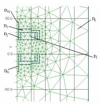
Fig.1 The integration domain for frontal symmetric couplings in normal environments
