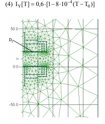
Fig. 3 The integration domain in the case of symmetric frontal couplings placed in magnetic powder and high temperature environments
